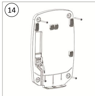
Screw the Plug-in base to the wall(x4)
