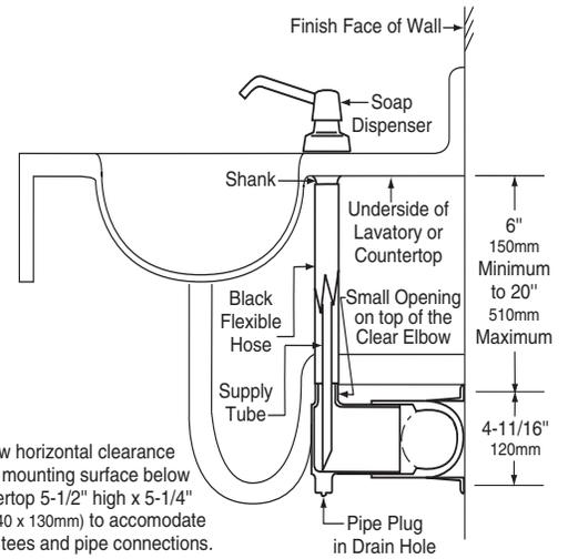
Allow horizontal clearance along mounting surface below countertop 5-1/2" high x 5-1/4" deep (140 x 130mm) to accommodate coupling tees and pipe connections.
