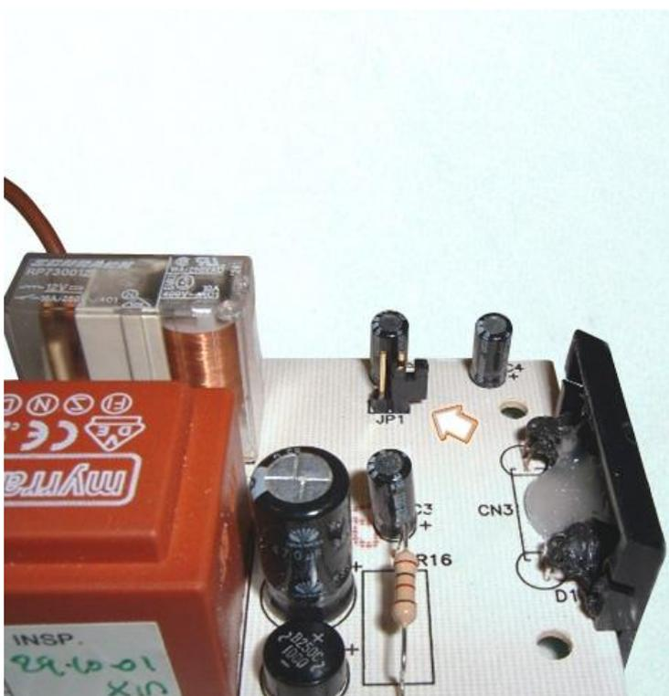
Position of the jumper at low sensitivity: detection distance between 15 and 20 cm.
