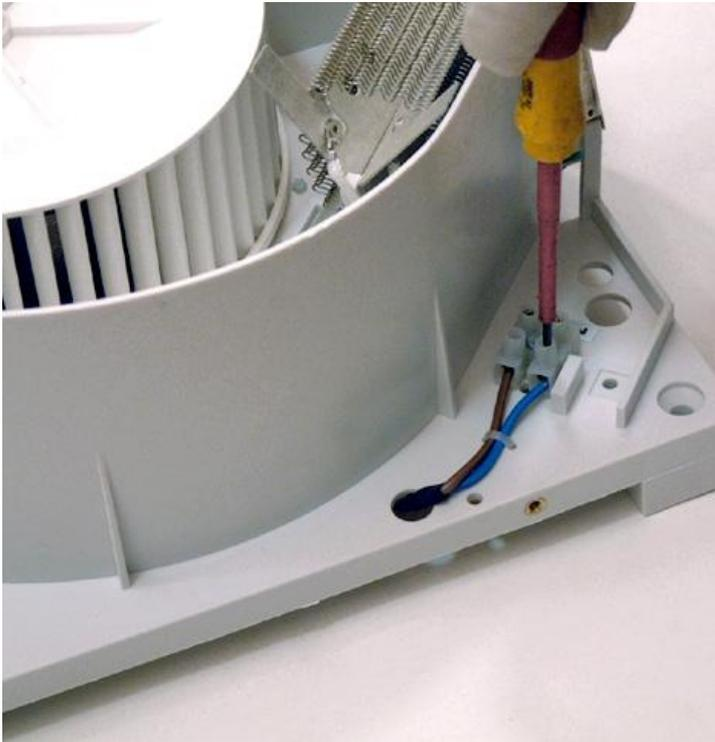
Disconnect the four cables; two from the motor (red and brown) and two from the heating element (white), from the terminal block of the electronic circuit board.
