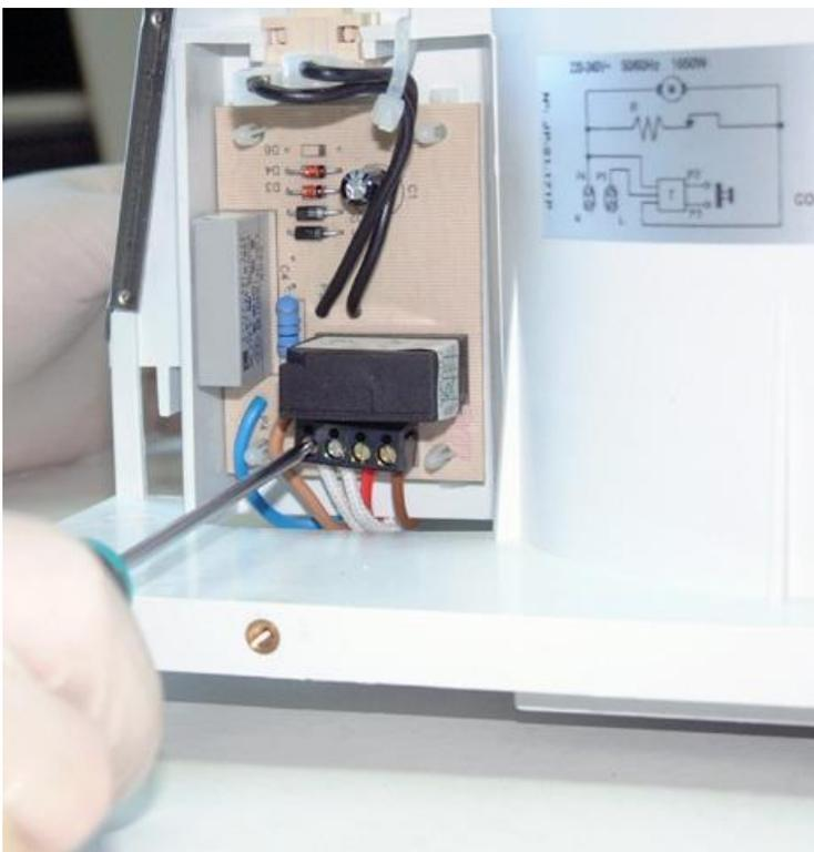
Disconnect the two timer cables that go to the button.
