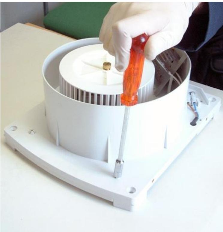
With a 7 mm hexagonal spanner loosen the screws located on the crosspiece of the base.
