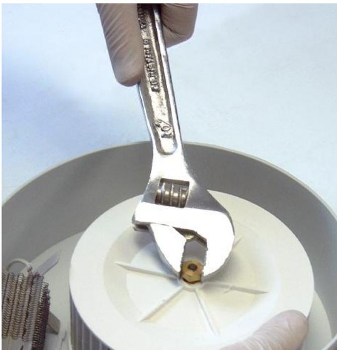
Using an 8 mm hexagonal spanner, separate the base from the rear cover by applying a slight pressure on the four clips.
