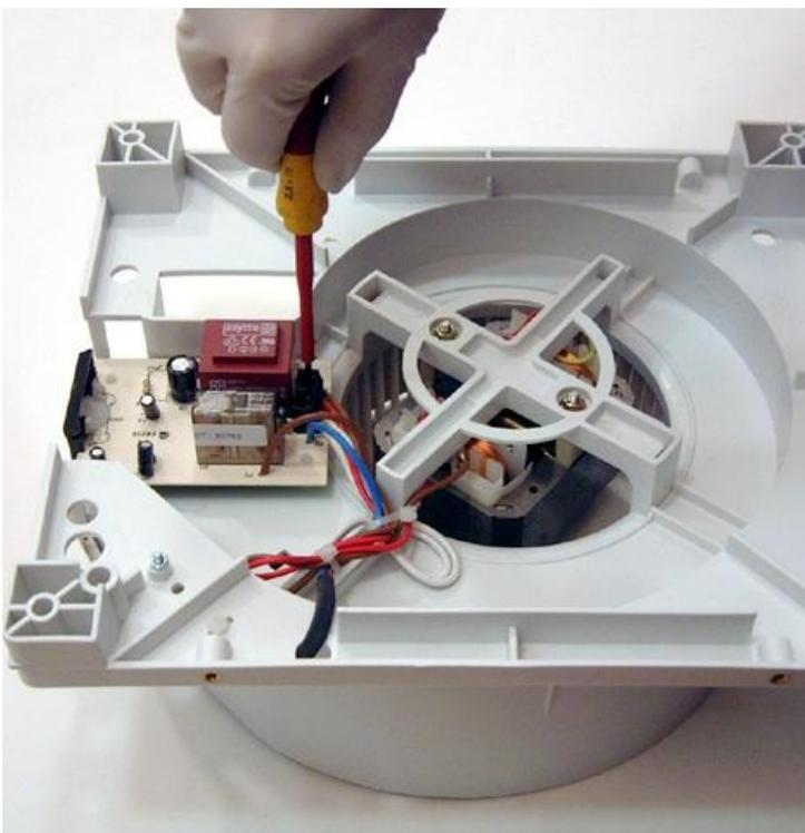
With a 7 mm hexagonal spanner loosen the screws located at the crosspiece of the base.
