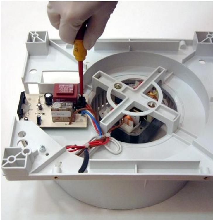
Remove the electronic circuit board from its housing, carefully freeing it from its four anchoring points and replace it. Fit it by following the previous steps in reverse order.
