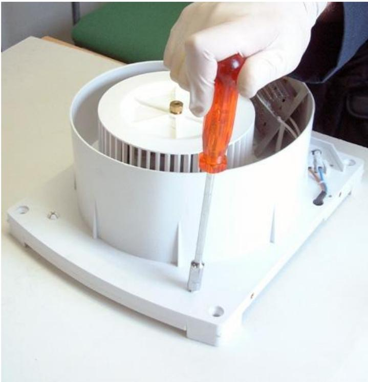
Disconnect the two cables from the heating element (white) that go to the terminal block of the electronic circuit board.
