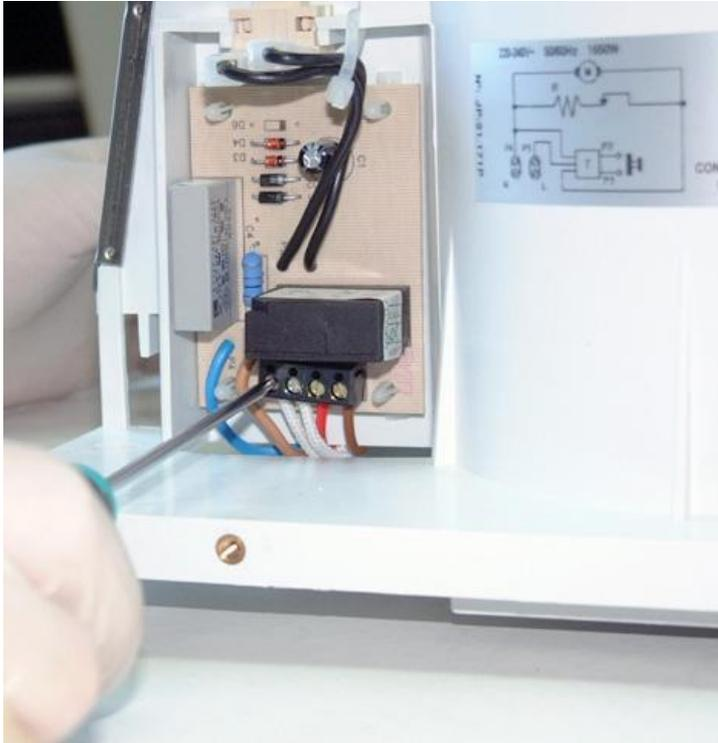
Remove the heating element from its location by bending the fastening clip and replace it. Fit it by following the previous steps in reverse order.
