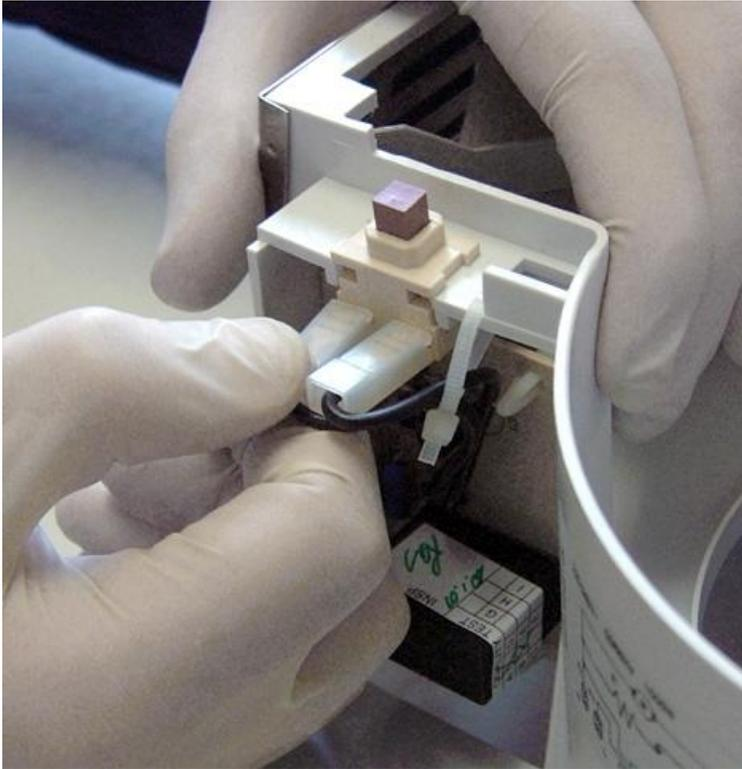
Remove the timer from its location, carefully freeing it from its four anchoring points using a flat-tipped tool and replace it.
