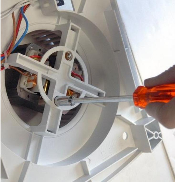
Remove the motor from its location and replace it. Fit it by following the previous steps in reverse order.
