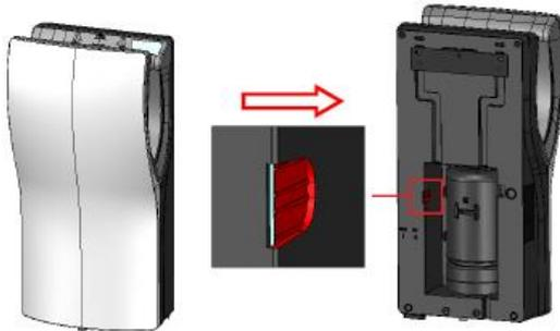
Break the flap on the rear side of the hand dryer base. Use a screwdriver and a hammer to do it more easily
