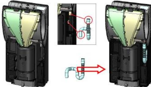
Introduce one end of the new tube through the new hole in the backside and fix the other side over the remaining part of the cut old tube using the provided flange
