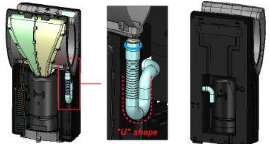
Confirm that the new tube maintains a "U" shape once assembled and connect the backside part of the tube to the waste pipe. Finally, assemble the frontal cover.
