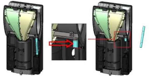
Disassemble the frontal cover and cut the original drain tube skim to the plastic union using a cutter
