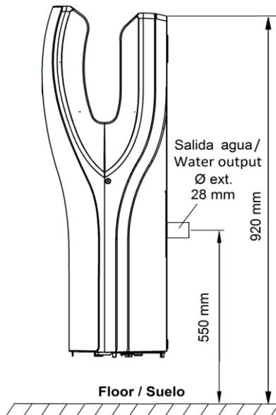
If the hand dryer is installed according to the installation instructions (upper back part of the dryer at 920 mm height), the main drain pipe installation should be approximately 450 mm from the water outlet height to the floor.
